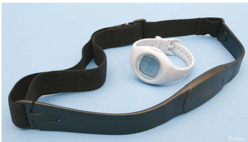
For example, the belt of a pulse counter sends the pulse rate to the display device held on the wrist using a low-power radio transmitter.
