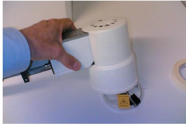
Fig. 4. Measuring a high-resolution alpha spectrum at ambient air pressure.
