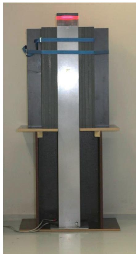
**Fig. 2.** 4"x4"x16" NaI detector moderated with PE.
