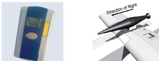
Fig. 5. A CsI gamma-ray spectrometer and TIKKA sampler.
