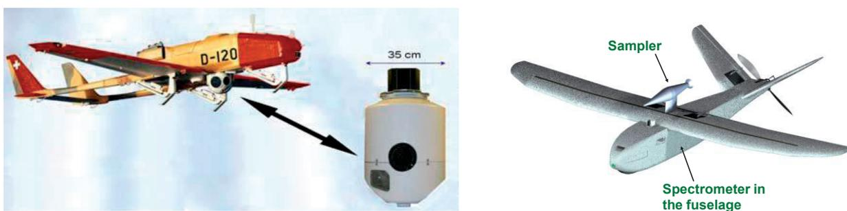
Fig. 1. Radiation detection instrumentation in Ranger mid-size UAV and in Patria MASS mini-UAV.
