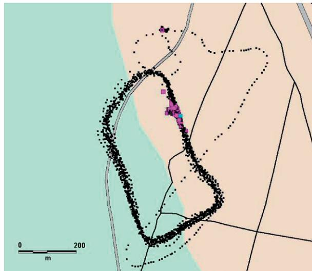
Fig. 4. Detecting a point source on the ground (coloured points). The route of the mini-UAV is shown as dots.
