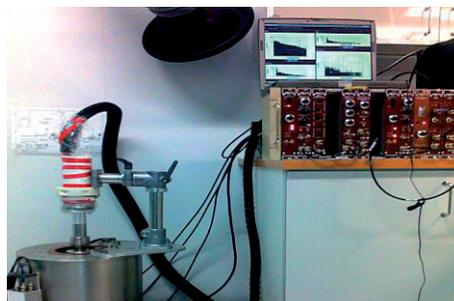
**Fig. 3.** The MiniPANDA system, based on alpha/beta/gamma coincidence counting, utilizes VASIKKA for data acquisition and storage.
