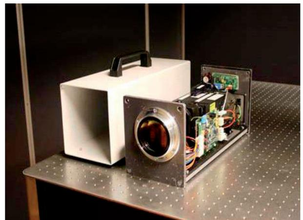
Fig. 2. HAUVA device for optical remote detection of alpha radiation.
