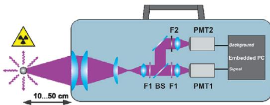
Fig. 4. Schematic model of signal and background measurement system in HAUVA.
