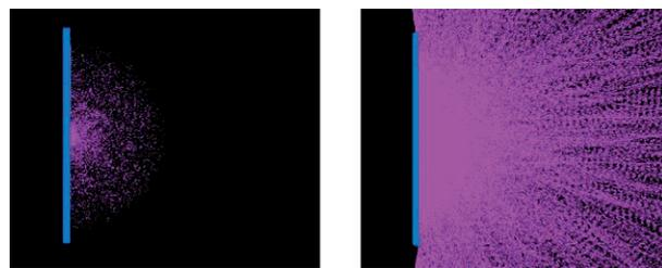
Fig. 5. Model of point alpha emitter on surface. a) Locations of ionization. b) Tracks of emitted fluorescence photons.
