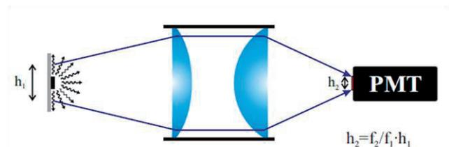
Fig. 1. Photomultiplier tube (PMT) and optics for collection of UV photons induced by a radioactive source emitting alpha particles.
