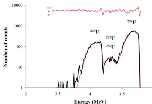
Fig. 4. Unfolding an alpha spectrum from particles containing U.
