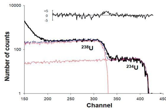
Fig. 5. Unfolding an alpha spectrum from a DU penetrator.
