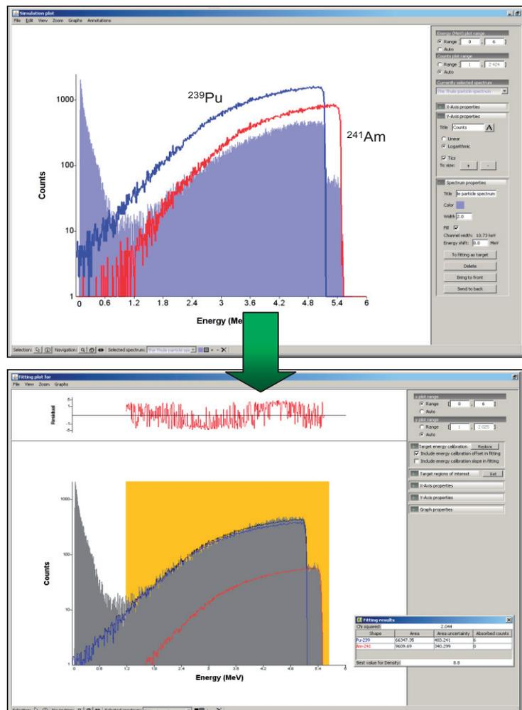
Fig. 1. Measured alpha spectrum from a nuclear bomb particle containing  $^{239}\text{Pu}$  and  $^{241}\text{Am}$  with simulated peak family shapes (at the top) and respective area-fitted shapes (bottom).
