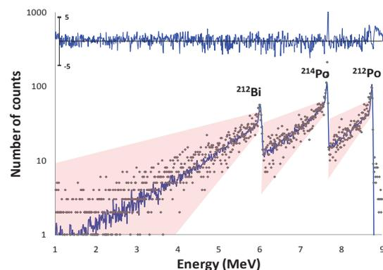
Fig. 3. Alpha spectrum from a glassfibre filter and fitted peaks of  $^{212}\text{Po}$ ,  $^{214}\text{Po}$  and  $^{212}\text{Bi}$ . The shaded areas illustrate the effect of varying penetration depth
