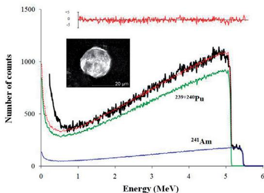
Fig. 2. Alpha spectrum from a nuclear bomb particle of diameter 25  $\mu\text{m}$  unfolded by AASIFIT.
